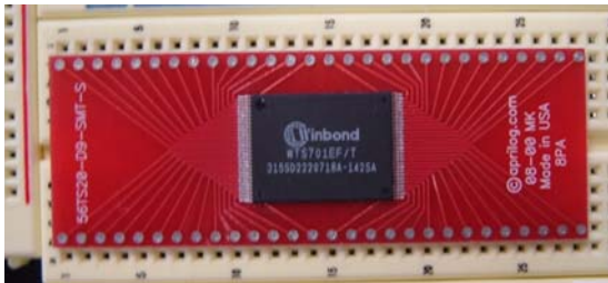
Figure 1, Speech Chip and DIP adapter.
