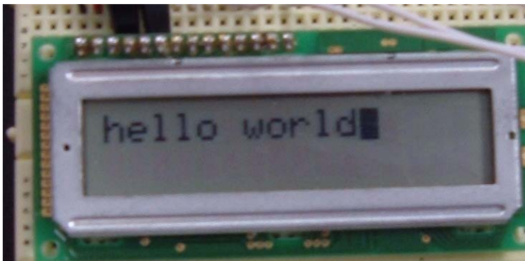
Figure 1, LCD screen displaying “hello world” as commanded by the microprocessor.
