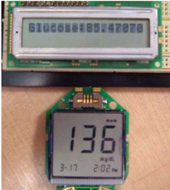
Figure 1: Photograph of the Actual Glucose Concentration to that of the Project Meter
