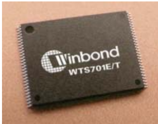
Figure 11: Winbond WTS701 Chip
